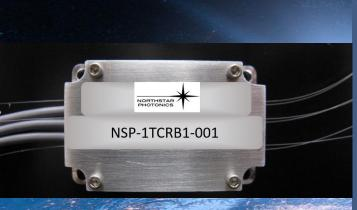
The Cerberus Three-channel Integrated Optical Circuit Assembly (IOCA) Phase Modulator is a custom module designed by Northstar Photonics, LLC for use in interferometric fiber optic gyroscope (IFOG) applications. This design incorporates three individual IOC assemblies into a single light-weight package that delivers our world-class performance with minimum cross-talk. The proprietary Northstar Photonics IOC technology has demonstrated lifetime in vacuum of more than 60 years.
